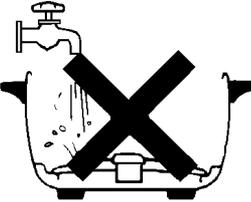
**DO NOT SPLASH WATER ONTO BODY.** Remember this is an electric appliance. Rice cooker and pot exterior must be clean and dry before use. Failure to follow this instruction will not only damage unit but create electrical hazard.
