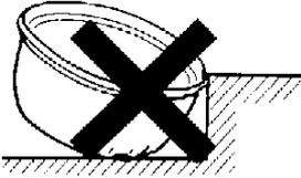
**DO NOT DENT POT** or use if for any other purpose. Changing the shape of the pot will cause the unit to shut off early, cook unevenly, or fail. Replace pot if dented.
