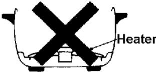
**DO NOT PLUG UNIT IN WITHOUT POT IN UNIT.** It can cause heater to deform. Deformed or damaged heaters must be replaced before further operation. Make sure to unplug unit before removing pot.
