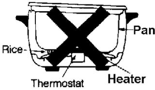
**KEEP THIS UNIT CLEAN.** Heater, thermostat, and pot must be clean if the unit is to operate properly. Rice, water, or anything else that is allowed onto heater will cause early shut off, uneven cooking, or unit damage. Pot exterior must also be clean.
