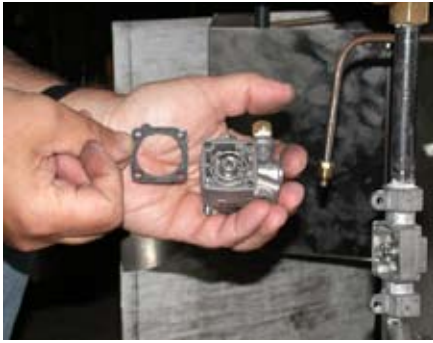
9. Install the new safety head with the new gasket provided (discard old gasket.)
