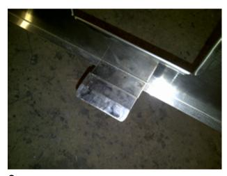
3 LATCH ON BOTTOM OF FRONT PANEL. PULL DOWN TO UNHOOK. THERE MAY BE SEVERAL OF THESE.
