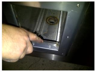
2 REMOVE SCREWS HOLDING SINK.
