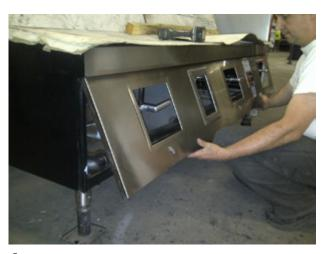
6 PUSH UP TO UNHOOK PANEL FROM TOP OF CHASSIS AND PULL AWAY FROM THE UNIT TO REMOVE PANEL.
