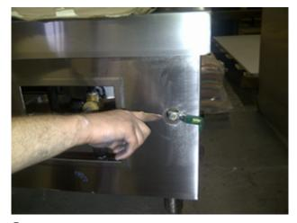
1 UNSCREW NUT AND REMOVE WATER VALVE HANDLE.
