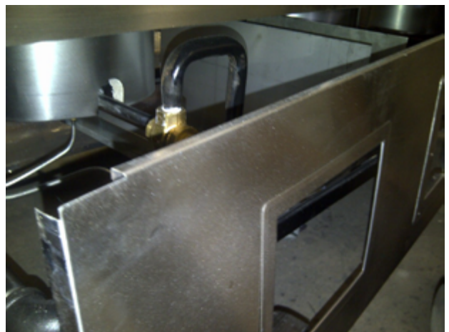
4 TOP PORTION OF PANEL IS HOOKED ONTO TOP OF CHASSIS.
