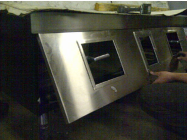
5 PULL BOTTOM PORTION OF PANEL AWAY FROM UNIT.
