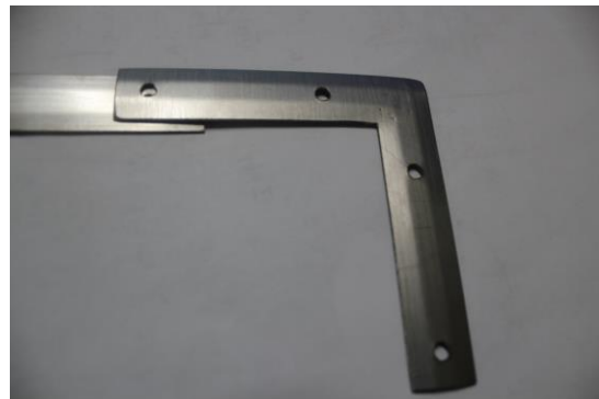
Figure 5 – Overlap of corner and side strips
