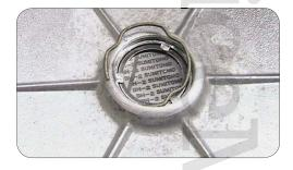
Pictured above: A sensor with it's retainingring removed.
