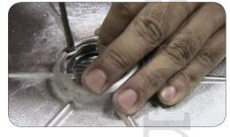
6) Place the sensing element into the pot, with the aluminum side facing into the pot, leaving the sensor exposed. Replace the retaining ring with a screwdriver.
