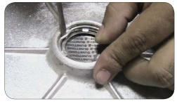
2) Use a flat head screwdriver to remove retaining ring, and replace the sensor.
