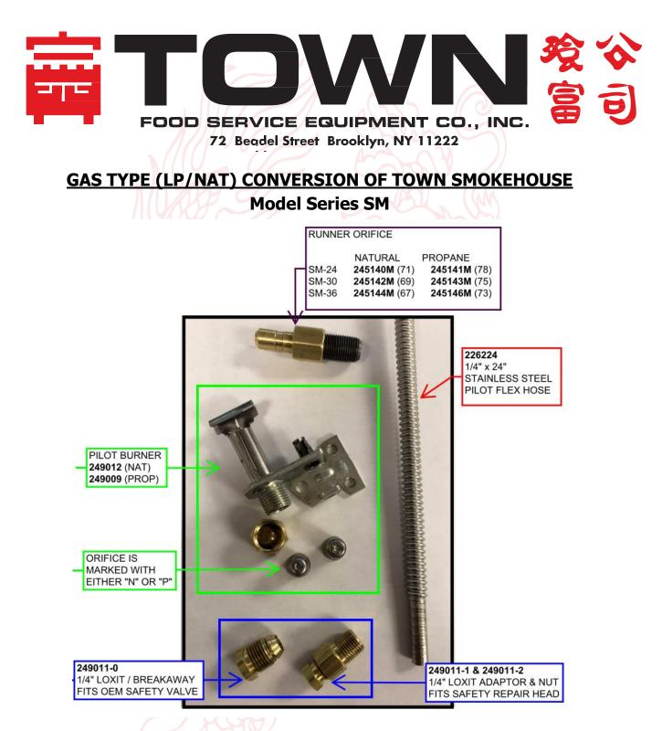
To convert the unit, the following parts need to be purchased: (1) pilot runner orifice, (1) safety pilot burner, (1) corrugated stainless steel pilot tube, appropriate safety valve fitting. Part numbers are bolded in the image above.
