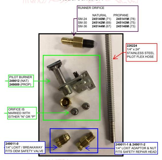
To convert the unit, the following parts need to be purchased: (1) pilot runner orifice, (1) safety pilot burner, (1) corrugated stainless steel pilot tube, appropriate safety valve fitting. Part numbers are bolded in the image above.
